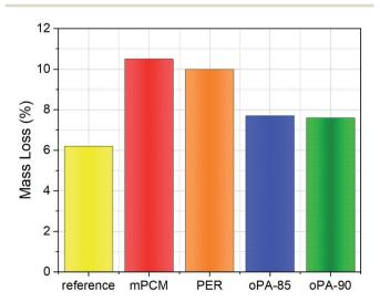
Fig. 6 Noncombustibility tests of concrete samples.
