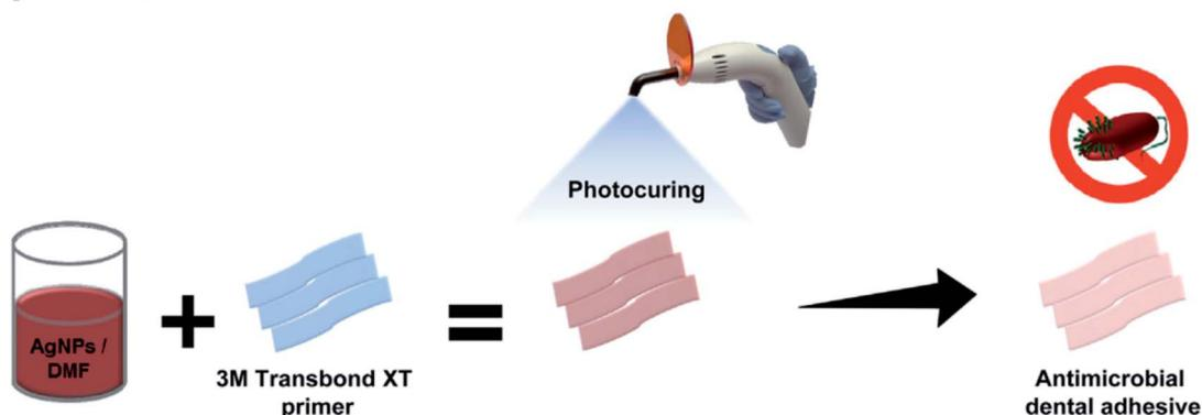
Fig. 8 Schematic illustration of the preparation of Ag NPs and the hybrid dental resin.<sup>149</sup>
