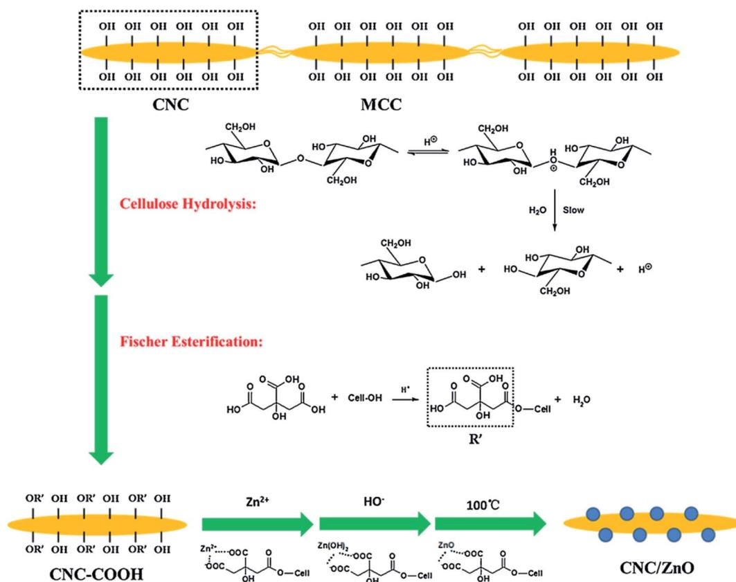
Fig. 9 The preparation route of cellulose nanocrystal/zinc oxide (CNC/ZnO) nano-hybrids.<sup>164</sup>
