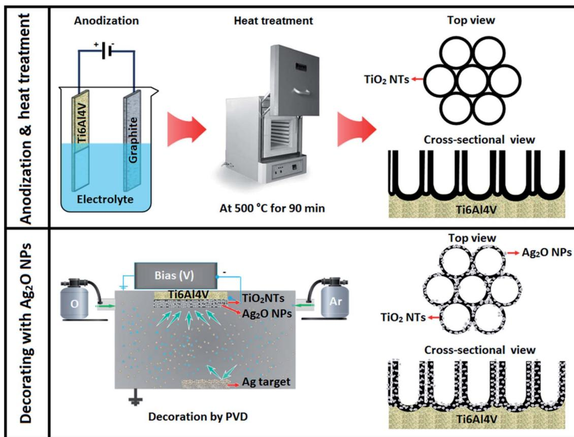
Fig. 3 Schematic representation of the anodization setup and the development of TiO<sub>2</sub> NTs as well as PVD decoration of Ag<sub>2</sub>O NPs on the nanotubular layer.<sup>122</sup>
