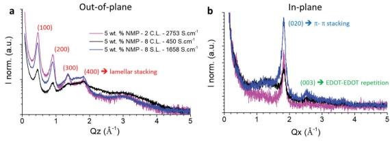
Fig. 4 (a) Out-of-plane and (b) in-plane diffractograms of PEDOT:OTf films synthetized with 5 wt% of NMP. The magenta curve is a thin film made of two continuous layers of 132 nm. The black and blue curves correspond respectively to eight continuous (2830 nm) and stacked layers (1168 nm) films. The crystallographic assignments in the out-of-plane and in-plane correspond to an orthorhombic lattice. 44
