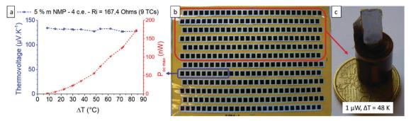
Fig. 5 (a) Thermovoltage and power density measured for a 9-thermocouples TEG module (b) picture of 312 spray-coated legs on a 25 µm thick polyimide foil (c) 3D TEG composed of 156 linked and rolled thermocouples ( $R_i = 2.9 \text{ k}\Omega$ ).
