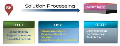
Fig. 31 Requirements of the active layer for OTFTs, oligo(p-phenylene vinylene) (OPVs), and OLEDs.
