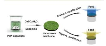
Fig. 91 CuSO<sub>4</sub>/H<sub>2</sub>O<sub>2</sub> triggered the rapid formation of PDA-based ultrathin selective layers with high uniformity and enhanced stability for both aqueous nanofiltration and organic nanofiltration. Reprinted from ref. 649 with permission. Copyright (2017) American Chemical Society
