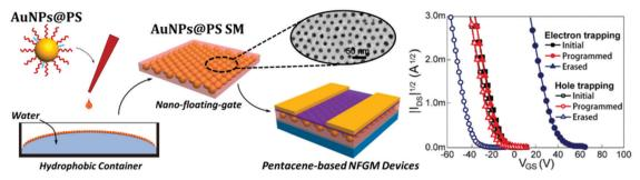
Fig. 72 Schematic illustration showing the strategy for fabricating AuNPs@PS SM through rapid liquid-liquid interface assembly on a convex water surface, and the design for NFGM devices based on a superlattice monomer. Adapted from ref. 532 with permission. Copyright (2018) from Wiley-VCH.
