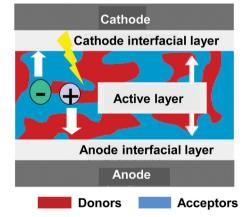
Fig. 24 Structure of a BHJ solar cell.
