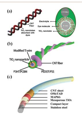
Fig. 98 Fiber-shaped solar cells with different active materials and architectures. (a) Fiber-shaped dye-sensitized solar cell twisted from Ti wire and CNT fiber. (b) Fiber-shaped polymer solar cell with a twisted structure. (c) Fiber-shaped PVSC with a coaxial structure. Reproduced from ref. 712 with permission. Copyright (2016) Wiley-VCH.
