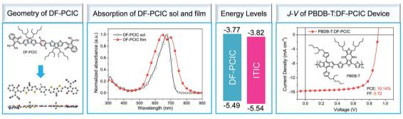
Geometry, absorption, and energy levels of DF-PCIC and device performance of PBDB-T:DF-PCIC-based OSCs.
