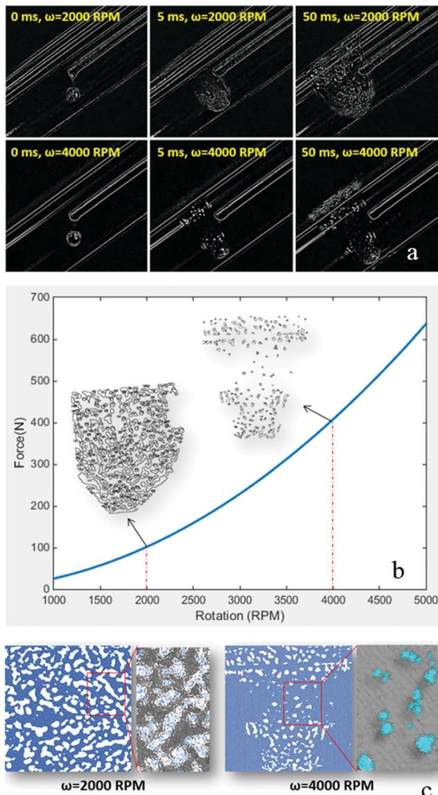
**Fig. 4** Modelling and schematic illustration of the formation of TPE nanoparticles at different rotational speeds. (a) Images captured by a high-speed camera at 2000 and 4000 rpm. (b) Modelling of resultant forces exerted on a TPE-THF drop after landing in rotating water in the VFD (insets: post-processed images indicating regions rich in TPE-THF that were formed after injection). (c) Schematic illustration of the formation of particles within regions rich in THF and encapsulated in water.
