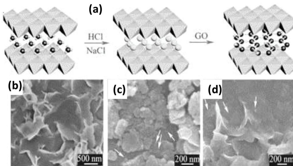
**Fig. 8** (a) Fabrication process of the NiFe-LDH/GO hybrids. (b–d) SEM images of NiFe-CO<sub>3</sub> LDHs, NiFe-Cl LDHs, and NiFe-LDH/GO hybrids. Reproduced and modified with permission from ref. 112. Copyright 2014, Wiley VCH.
