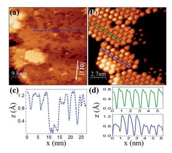
Fig. 2 (a) STM topographic image of  $\approx 0.4$  ML of  $C_{60}F_{48}$  on Cu (111) at RT; I = 190 pA, bias = +1.0 V. (b) Magnified image; I = 190 pA, V =+1.8 V. (c and d) Profiles along the segments of respective color in (a and b). The crystallographic directions were determined from LEED (see Experimental details). The molecular hexagonal lattice is aligned with respect to the main crystallographic directions of the Cu(111) surface forming a  $(4 \times 4)R0^{\circ}$  superstructure.
