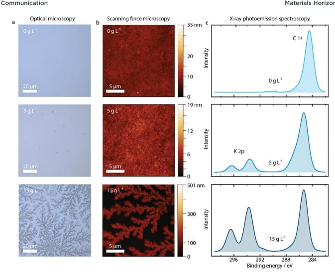
Effect of KCl incorporated within the PEDOT:PSS layers. The optical microscopy (a) and scanning force microscopy images (b) of the PEDOT:PSS films show a clear influence of the concentration of KCl additive (0, 5, 15 g  $L^{-1}$ ) on the film morphology. XPS spectra (c) indicate that as the KCl concentration increases within the PEDOT:PSS films, so does the K 2p peak (doublet at 295 eV) corresponding to the added KCl. The C 1s peak (285 eV) corresponding to the PEDOT:PSS surface shows no change.
