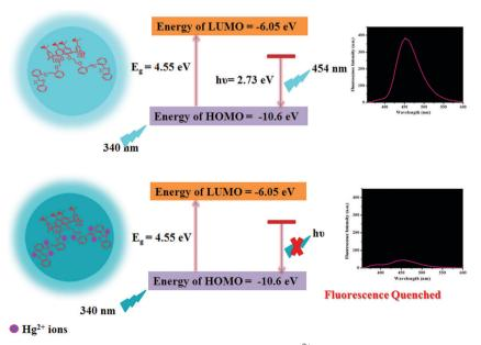
Scheme 2 Schematic representation of the plausible mechanism for the binding of Hg<sup>2+</sup> ions with the as-synthesized CDs.
