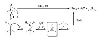
Scheme 1  $I_2$ -Mediated mechanism of Sn(II) oxidation in DMSO. A possible intermediate species, iododimethylsulfonium iodide, is highlighted inside the square.
