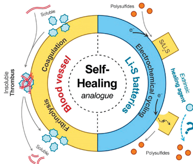
Fig. 25 Schematic of healing mechanism for sulfur particle cathodes. (left side) Simplified schematic of coagulation cascade toward formation of thrombus (blood clot) and fibrinolysis of thrombus into soluble fibrin fragments, which are modulated by two trypsins: thrombin and plasmin; (right side) schematic of deposition and dissolution of micrometer-sized sulfur/Li 2 S particles with limited electrical contact, hindering full electrochemical utilization. To enable the stable and reversible utilization, a complementary route is introduced, through chemical reactions between an extrinsic healing agent in solution and insoluble sulfur compounds. Reprinted with permission from ref. 413. Copyright 2017 American Chemical Society.
