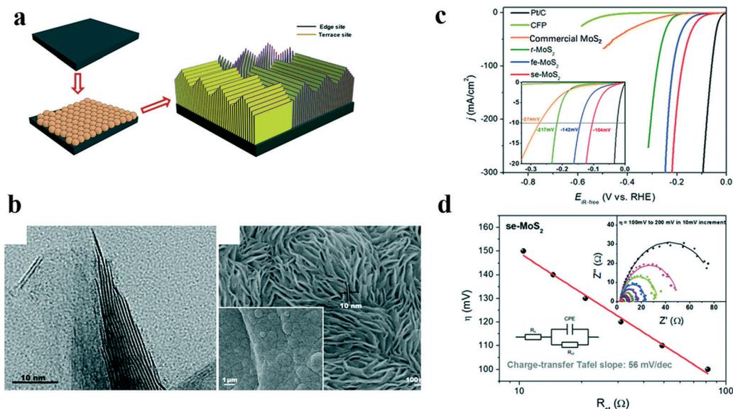
Fig. 6 Effects of high index faces on the catalytic performance of MoS<sub>2</sub>.<sup>54</sup> (a) Schematic illustration of stepped edge surface-terminated MoS<sub>2</sub> arrays (se-MoS<sub>2</sub>), (b) HRTEM image of the se-MoS<sub>2</sub> layers showing that the crystal fringes of the S–Mo–S layers along the edge are stepped, (c) polarization curves and (d) charge-transfer Tafel plots of se-MoS<sub>2</sub> and control catalysts.
