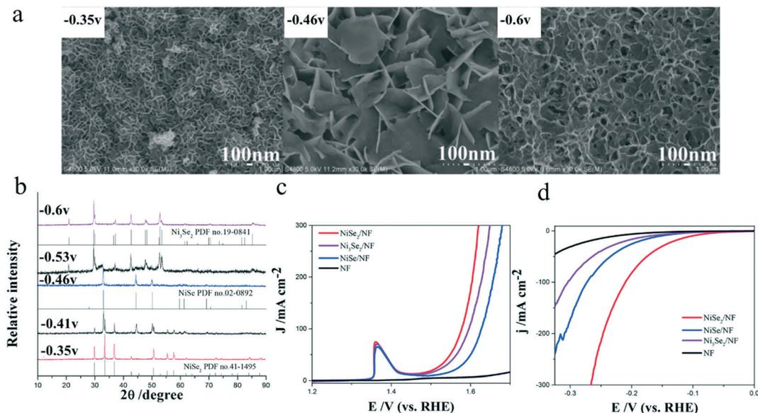
**Fig. 3** Controlled synthesis of nickel selenides in different crystal phases.<sup>22</sup> (a) FESEM images of the as-prepared nickel selenides with different crystal phases taken at various deposition potentials:  $-0.35$ ,  $-0.46$ , and  $-0.60$  V; (b) XRD patterns of the nickel selenides; (c and d) polarization curves of these nickel selenides for (c) HER and (d) OER.
