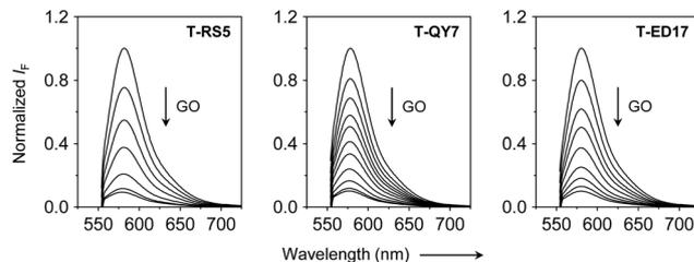
**Fig. 3** Fluorescence titration of **T-RS5**, **T-QY7** and **T-ED17** (0.5  $\mu$ M) with increasing GO (from top to bottom curve: 0–12  $\mu$ g mL<sup>-1</sup> for **T-RS5**, 0–56  $\mu$ g mL<sup>-1</sup> for **T-QY7** and 0–38  $\mu$ g mL<sup>-1</sup> for **T-ED17**, respectively). All measurements were carried out in PBS (0.01 M, pH 7.4, containing 1% DMSO, v/v) with an excitation of 525 nm.
