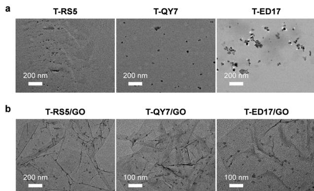
**Fig. 2** Transmission electron microscopic images of (a) **T-RS5**, **T-QY7** and **T-ED17** (10  $\mu$ M), and (b) **T-RS5/GO**, **T-QY7/GO** and **T-ED17/GO** (peptide/GO = 10  $\mu$ M/40  $\mu$ g mL<sup>-1</sup>).
