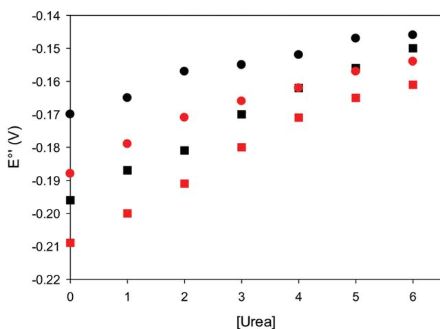
**Fig. 7** Urea-induced changes in  $E^{\circ'}$  for the M80A (circles) and M80AY67A (squares) variants of *S. cerevisiae* iso-1 cytochrome c at 5 °C (red) and 25 °C (black). Working electrode: polycrystalline gold wire functionalized with 4-mercapto-pyridine. 10 mM phosphate buffer plus 100 mM sodium perchlorate, pH 7.2.
