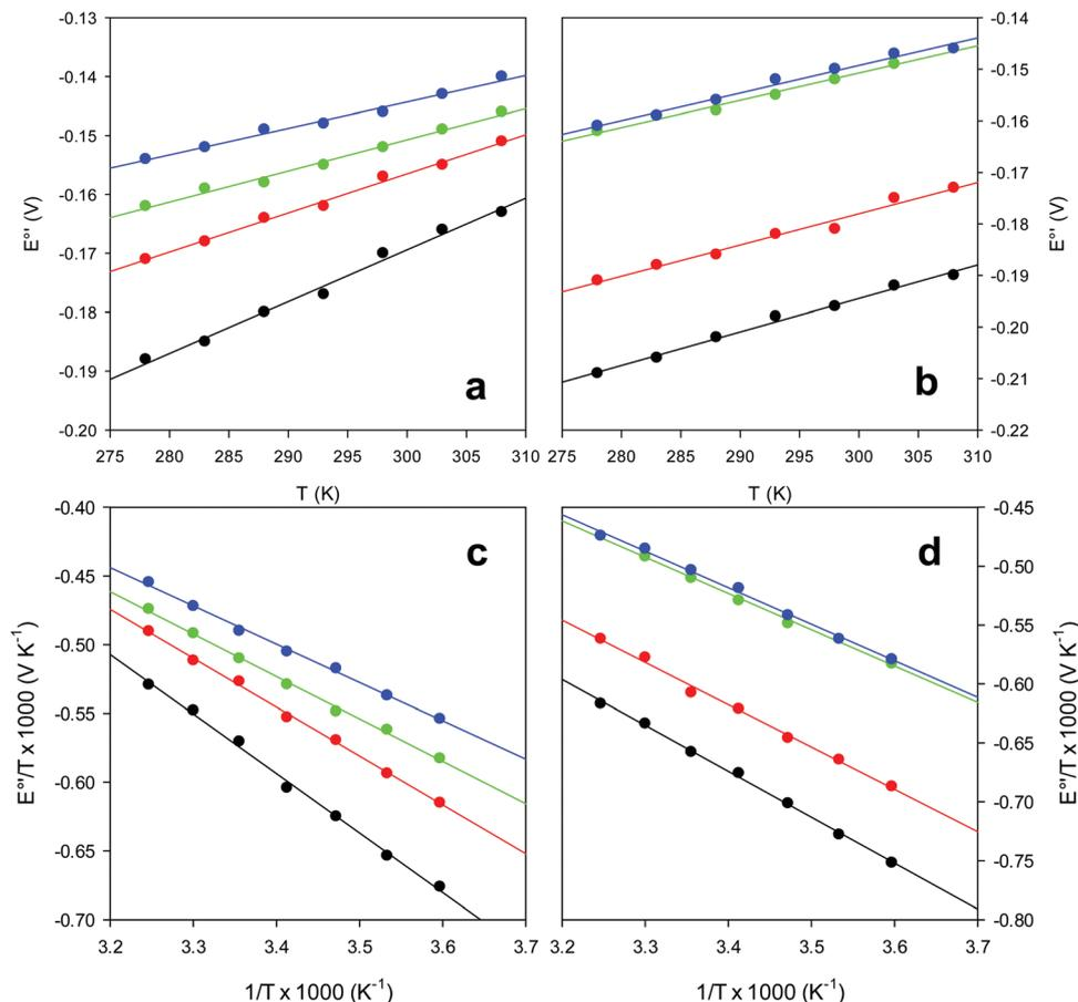
**Fig. 8** Plot of  $E^{\circ}$  versus  $T$  and  $E^{\circ}/T$  versus  $1/T$  for the M80A (a and c) and the M80A/Y67A (b and d) variants of yeast iso-1-cytochrome c in the presence of urea 0 M (black), 2 M (red), 4 M (green) and 6 M (blue), in 10 mM phosphate buffer plus 100 mM sodium perchlorate, pH 7.2. Solid lines are least-squares fits to the data points.
