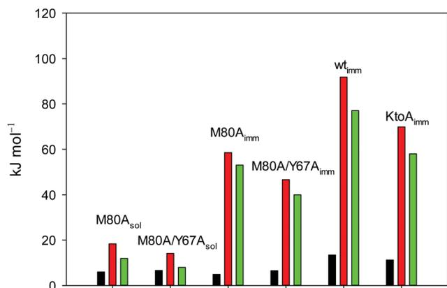
**Fig. 12** Histograms depicting the thermodynamic parameters of urea-induced unfolding for yeast iso-1-cytochrome *c* and its variants in solution and in the immobilized state reported in Table 4. Black, red and green bars correspond to  $\Delta G_u^{\circ\text{H}_2\text{O}}$ ,  $\Delta H_u^{\circ\text{H}_2\text{O}}$  and  $T(5\text{ °C})\cdot\Delta S_u^{\circ\text{H}_2\text{O}}$  values, respectively.
