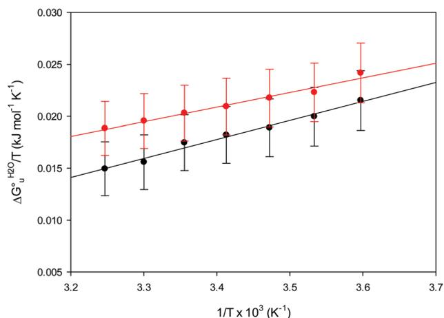
**Fig. 11** van't Hoff plots for the urea-induced unfolding of the M80A (black) and the M80A/Y67A (red) variants of yeast iso-1-cytochrome c in 10 mM phosphate buffer plus 10 mM sodium perchlorate, pH 7.2. Solid lines are least-squares fits to the data points.
