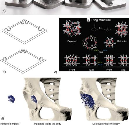
Fig. 1 (a) A number of AM orthopaedic implants (reprinted from ref. 46 with permission from Elsevier, Copyright 2018). (b) The basic bi-stable elements used for the design of multi-stable deployable implants.<sup>38</sup> (c) A deployable implant made through an arrangement of bi-stable implants.<sup>38</sup> (d) A schematic demonstration of the concept of deployable implants.<sup>38</sup>
