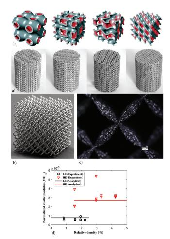
Fig. 3 (a) Some examples of the meta-biomaterials designed using different types of triply periodic minimal surfaces and fabricated using selective laser melting. 63,115 (b) Pentamode metamaterials made from Ti-6Al-4V<sup>65</sup> and (c) the double-cone shape of their struts.<sup>65</sup> (d) The Ashby's law between relating relative density to the mechanical properties of cellular structures breaks down in the case of pentamode metamaterials.65
