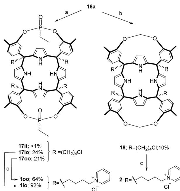
Scheme 2 Synthetic schemes for the preparation of the cavitands **17** and **18** and their water soluble derivatives **1** and **2**. <sup>a</sup>Reaction conditions: (a) EtPOCl<sub>2</sub>, Et<sub>3</sub>N in THF; (b) K<sub>2</sub>CO<sub>3</sub>, MeBrCl in DMSO; (c) excess pyridine and heat.
