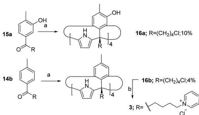
Scheme 1 Synthetic schemes for the preparation of the calix[4]pyrroles **16a** and **16b** and the water soluble derivative **3**. Reaction conditions: (a) MeNBu<sub>3</sub>Cl, HCl (4 M dioxane), pyrrole in DCM; (b) excess pyridine and heat.
