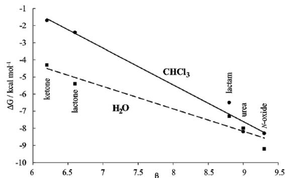
**Fig. 8** Plot of  $\Delta G$  vs. H-bonding acceptor capabilities ( $\beta$ ) for the inclusion complexes of the five 6-membered cyclic guest with **100** (squares, H<sub>2</sub>O dashed-line) and **1700** (circles, CHCl<sub>3</sub> solid-line) receptors. This graphical analysis serves to illustrate the hydrophobic effect contribution to binding.
