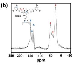
Fig. 1 (a) FTIR and (b) C-NMR spectra of COPN-1
