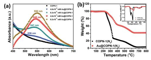
Fig. 4 (a) UV spectra of COPN-1 and Au@COPN-1 at different concentration ( $4.6 \times 10^{-4}$ ,  $9.2 \times 10^{-4}$ ,  $4.6 \times 10^{-3}$  and  $9.2 \times 10^{-3}$  mM Au) (b) TGA thermograms of COPN-1 and Au@COPN-1 ( $4.6 \times 10^{-3}$  mM Au) in N<sub>2</sub>.
