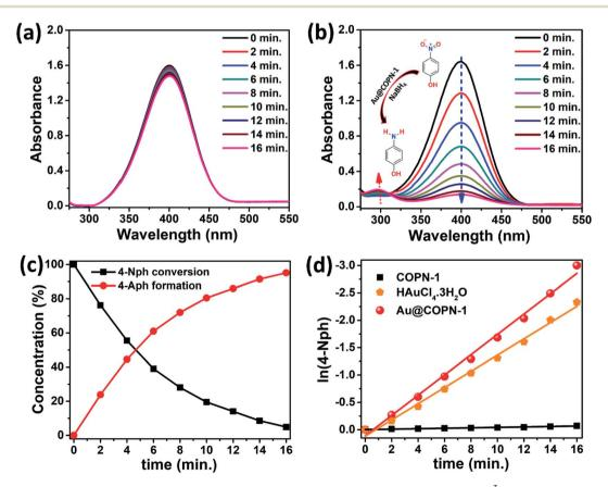
Fig. 5 Catalytic reduction of 4-nitrophenol by using NaBH<sub>4</sub>, (a) COPN-1, (b) with Au@COPN-1 ( $4.6 \times 10^{-3}$  mM Au), (c) kinetics of reduction process of 4-Nph solution (4-Aph formation) and (d) fitted data of the pseudo-first-order kinetics (Au@COPN-1, HAuCl<sub>4</sub>·3H<sub>2</sub>O, and COPN-1).
