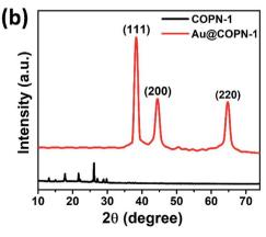
Fig. 2 (a) UV spectra and (b) XRD Pattern of COPN-1 and Au@COPN-1 ( $4.6 \times 10^{-3}$  mM Au).
