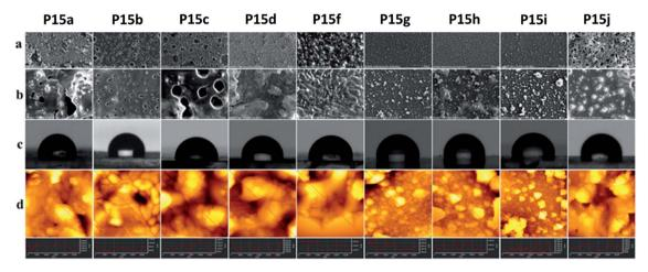
Fig. 2 SEM (a) 1.000×, (b) 10.000×; (c) contact angle, CA; (d) AFM topography images and surface cross section analyses of P15a-P15j
