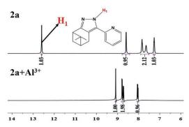
Fig. 5 <sup>1</sup>H NMR spectra changes in 2a with the addition of Al<sup>3+</sup>.
