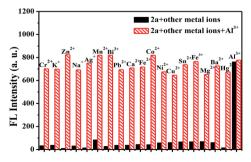
Fig. 2 Fluorescence intensity of 2a (5.0  $\times$  10<sup>-6</sup> M) in buffer solution (EtOH/HEPES buffer, v/v = 6/4, 10 mM HEPES, pH = 7.4) and its complexes with  ${\rm Al}^{3+}$  (5.0  $\times$   $10^{-5}$  M) in the presence of various metal ions (5.0  $\times$  10<sup>-5</sup> M),  $\lambda_{ex} = 330$  nm.
