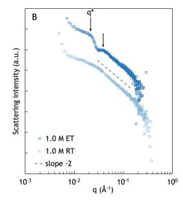
Fig. 4 SAXS spectra of PNIPAM-b-PDMAEMA and PNIPAM-b-PAA-b-PNIPAM in 0.5 M (A) and 1.0 M (B) NaCl at 27 °C (RT) and 67 °C (ET). As a guide to the eye, a dashed line is displayed to indicate a slope of –2. The presented data were corrected for solvent contributions and plotted on a log-log scale. Scattering intensities of the ET data were adjusted for clear display.
