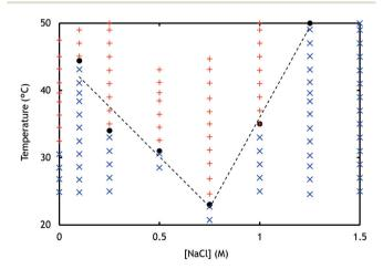
Fig. 2 Light scattering was used to determine the  $T_{cp}$  of samples containing PNIPAM-b-PDMAEMA and PNIPAM-b-PAA-b-PNIPAM with varying concentrations of NaCl. The results were used to create a phase diagram; the blue crosses represent a one phase system, and the red plusses represent an aggregated system. The dotted lines represent the phase boundary that was deduced from the observed  $T_{cp}$ s (black dots).
