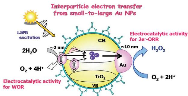
Scheme 4 Schematic representation of  $\text{H}_2\text{O}_2$  synthesis from water and O<sub>2</sub> by the BM-Au/TiO<sub>2</sub> plasmonic photocatalyst.
