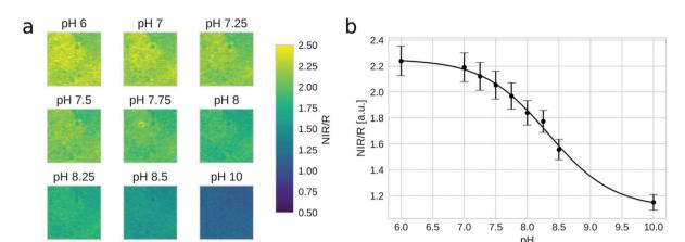
Fig. 6 Imaging of the pH distribution with the dual chip RGB/NIR camera. (a) False-color images for the fluorescence ratio (NIR/red channel) for the sensor material between pH 6 and 10. (b) The fit of the corresponding response curve with the Boltzmann sigmoid function.
