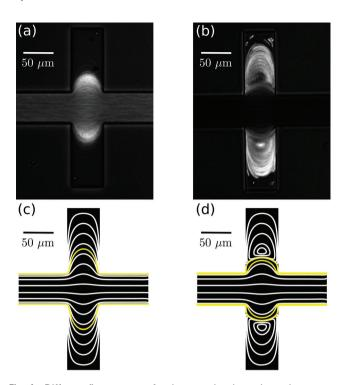
Fig. 4 Different flow patterns for the same in-plane channel geometry, but different channel depths of  $h=20~\mu m$  (a, c) and  $h=40~\mu m$  (b, d). Panels (a–b) show the standard deviation of microfluidic experiments whereas panels (c–d) illustrate the streamlines of corresponding creeping flow simulations.
