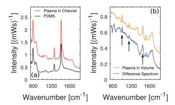
Fig. 8 NIR Raman spectroscopy of blood plasma in a microfluidic channel with 3 minutes integration time. (a) Fluorescent and Raman scattering from blood plasma are superimposed by the out-off focus Raman scattering by PDMS. (b) A scaled subtraction of the PDMS Raman signature from the spectrum corrects for the PDMS background and restores the pure spectrum of blood plasma.
