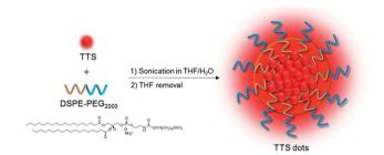
Fig. 3 Schematic illustration of AIE dot fabrication.
