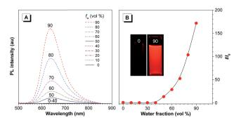
Fig. 2 (A) PL spectra of TTS in THF/water mixtures with different water fractions ( $f_{\rm w}$ ). (B) Plot of the relative PL intensity ( $I/I_0$ ) versus the composition of the THF/water mixture of TTS.  $I_0$  = emission intensity in pure THF solution. Concentration: 10  $\mu$ M; excitation wavelength: 480 nm. Inset: fluorescence photographs of TTS in THF ( $f_{\rm w}=0$ %) and THF/water mixture with  $f_{\rm w}=90$ % taken under 365 nm UV illumination.
