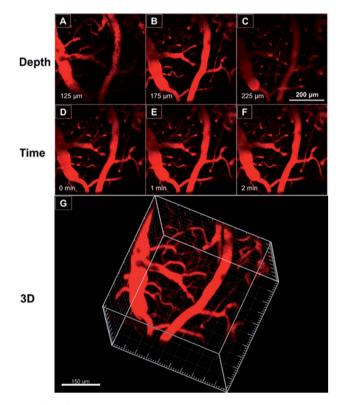
Fig. 8 (A–C) Representative two-photon fluorescence images of the blood vessels of a mouse brain, 0.5 h after injection of the TTS dots, at different penetration depths. (D–F) Representative time-lapse images of the blood vessels of a mouse brain, 0.5 h after injection of the TTS dots, at different monitoring time points and at a depth of 200 μm. Scale bar: 200 μm. (G) The constructed 3D image of the blood vessels of the mouse brain, 0.5 h after injection of the TTS dots. Scale bar: 150 μm.
