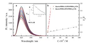
Fig. 9 (a) Fluorescence spectral response of quartz/PDDA-G/(PSS/PDDA)<sub>3</sub>/CDs SAMs toward Tc at different concentrations in 10 mM PB buffer of pH 6.8. (Inset graph shows the ratio  $F/F_0$  of fluorescence intensity varied with concentration of Tc). (b) Relationship curves between  $F_0/F$  of SAMs and Tc concentration.
