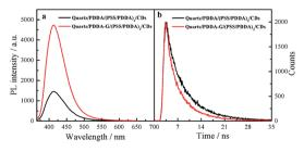
Fig. 4 Fluorescence spectra (a) and fluorescence decay curves (b) of quartz/PDDA/(PSS/PDDA)3/CDs SAMs and quartz/PDDA-G/(PSS/ PDDA)3/CDs SAMs
