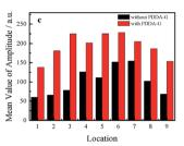
**Fig. 5** Fluorescence microscopy images of (a) quartz/PDDA/(PSS/PDDA)<sub>3</sub>/CDs SAMs and (b) quartz/PDDA-G/(PSS/PDDA)<sub>3</sub>/CDs SAMs. (c) Confocal fluorescence values of quartz/PDDA/(PSS/PDDA)<sub>3</sub>/CDs SAMs and quartz/PDDA-G/(PSS/PDDA)<sub>3</sub>/CDs SAMs with different matching locations.
