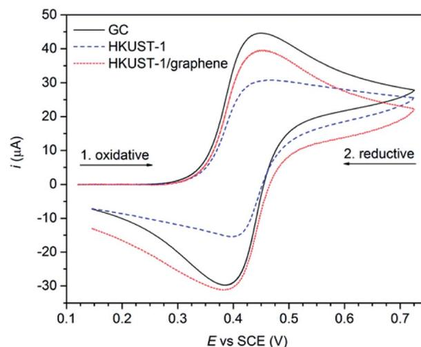
Fig. 7 CV measurements (recorded using a Ag/AgI reference electrode in 0.01 M TBA·BF<sub>4</sub>/acetonitrile, sweep rate: 0.1 V s<sup>-1</sup>) on a blank GC plate (black), a HKUST-1-covered GC plate (blue) and a composite film on GC (red) using 2 mM Fc as redox probe. These curves were obtained applying baseline removal and iR compensation to the original voltammograms (see Fig. S13†).
