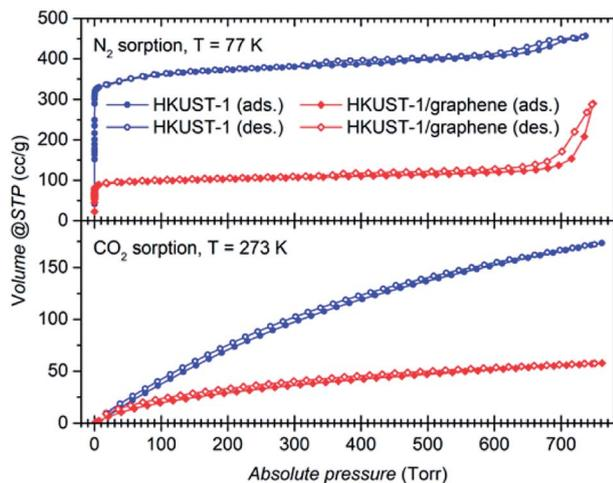
Fig. 5 (Top) Adsorption (filled symbols) and desorption (open symbols) curves at 77 K for  $N_2$  over bulk HKUST-1 (blue) and over the composite (red). (Bottom) adsorption and desorption curves for  $CO_2$  at 273 K of the same samples. The isotherms show higher adsorption capacity of the bare MOF compared to HKUST-1/graphene.
