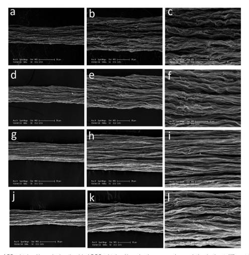
Fig. 6 SEM images of GFs obtained by reducing the dried GOFs obtained by using isopropanol coagulation baths at different temperatures under different magnifications (500×, 1000× and 2000×): (a-c) GF@35°-IPA; (d-f) GF@25°-IPA; (g-i) GF@15°-IPA; (j-l) GF@5°-IPA;
