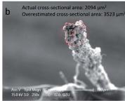
Fig. 3 (a) The paper frames used during the tensile tests; (b) SEM image of GOF@25°-IPA sample after the rupture during the tensile test to calculate their cross-section.
