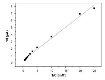
Fig. 7 The Lineweaver-Burk plot of the PEDOT-NFs/GOx-3 biosensor
