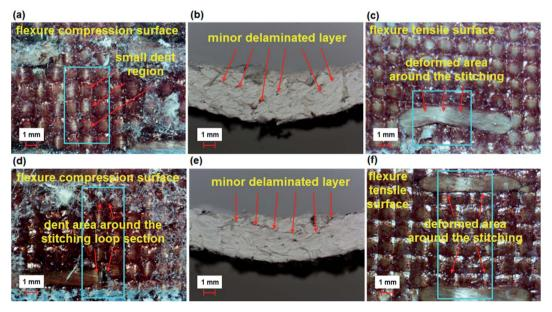
Fig. 12 Warp directional flexure failure in various multistitched 3D p-aramid/phenolic MWCNT composites. (a) Stitched top face (TB-TS); (b) stitched cross-section (TB-TS); (c) stitched bottom face (TB-TS); (d) stitched/nano top face (TB-TS-N); (e) stitched/nano cross-section (TB-TS-N) and (f) stitched/nano bottom face (TB-TS-N) (optical microscope, magnification  $\times$ 6.7).
