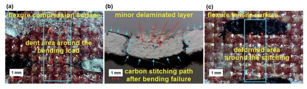
Fig. 13 Warp directional flexure failure in PAN carbon nanostitched p-aramid/phenolic MWCNT composites. (a) Stitched/nano top face (TB–CS–N); (b) stitched/nano cross-section (TB–CS–N); (c) stitched/nano bottom face (TB–CS–N) (optical microscope, magnification  $\times$ 6.7).
