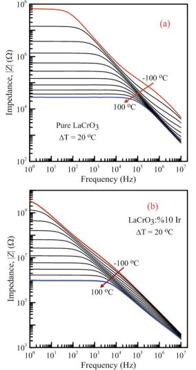
the temperature range from  $-100\,^{\circ}\text{C}$  to  $100\,^{\circ}\text{C}$  with steps of  $20\,^{\circ}\text{C}$ , (a) pure LaCrO<sub>3</sub> and (b) LaCr<sub>0.90</sub>Ir<sub>0.10</sub>O<sub>3</sub>.
