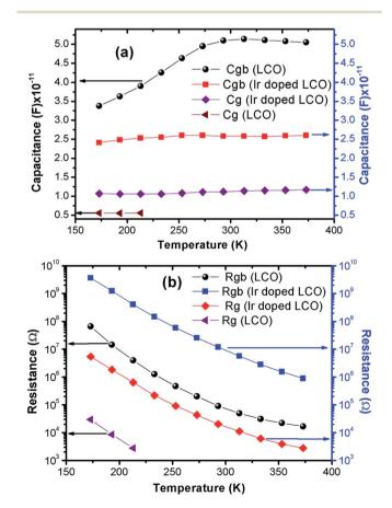
Fig. 12 Temperature dependent (a) capacity and (b) resistance plots of grain and grain boundary for LCO and Ir doped LCO.
