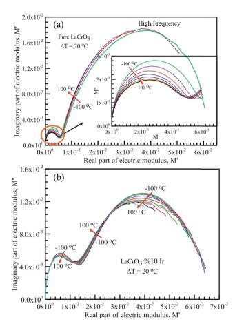
Fig. 8 Frequency dependent-electrical modulus plane plots, the imaginary M'' versus real M' in the temperature range from  $-100\,^{\circ}\text{C}$  to  $100\,^{\circ}\text{C}$  with steps of  $20\,^{\circ}\text{C}$ , (a) pure LaCrO<sub>3</sub>, inset: low frequency data of the complex electric modulus plane plot of the pure LCO sample, and (b) LaCr<sub>0.90</sub>Ir<sub>0.10</sub>O<sub>3</sub> sample.
