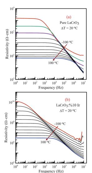
Fig. 15 Frequency dependence of the resistivity of both samples in the temperature range from  $-100~^{\circ}\text{C}$  to  $100~^{\circ}\text{C}$  with steps of  $20~^{\circ}\text{C}$ , (a) pure LaCrO<sub>3</sub> and (b) LaCr<sub>0.90</sub>Ir<sub>0.10</sub>O<sub>3</sub>.
