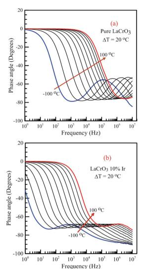
Fig. 14 Frequency dependence of the phase angle of both samples in the temperature range from -100 °C to 100 °C with steps of 20 °C, (a) pure LaCrO<sub>3</sub> and (b) LaCr<sub>0.90</sub>Ir<sub>0.10</sub>O<sub>3</sub> samples.
