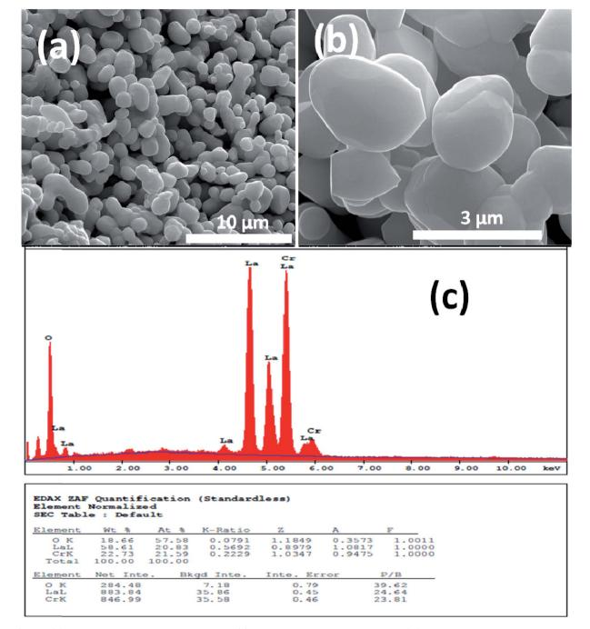
Fig. 1 (a and b) SEM images with different magnification (c) EDX analysis results for the pure LaCrO<sub>3</sub> powders, respectively.
