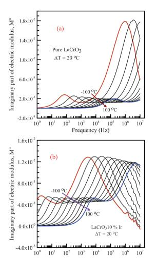
Fig. 7 Frequency dependence plots of the imaginary part of electrical modulus, M'' in the temperature range from  $-100~^{\circ}\text{C}$  to  $100~^{\circ}\text{C}$  with steps of  $20~^{\circ}\text{C}$ , (a) pure LaCrO<sub>3</sub> and (b) LaCr<sub>0.90</sub>|r<sub>0.10</sub>O<sub>3</sub>.
