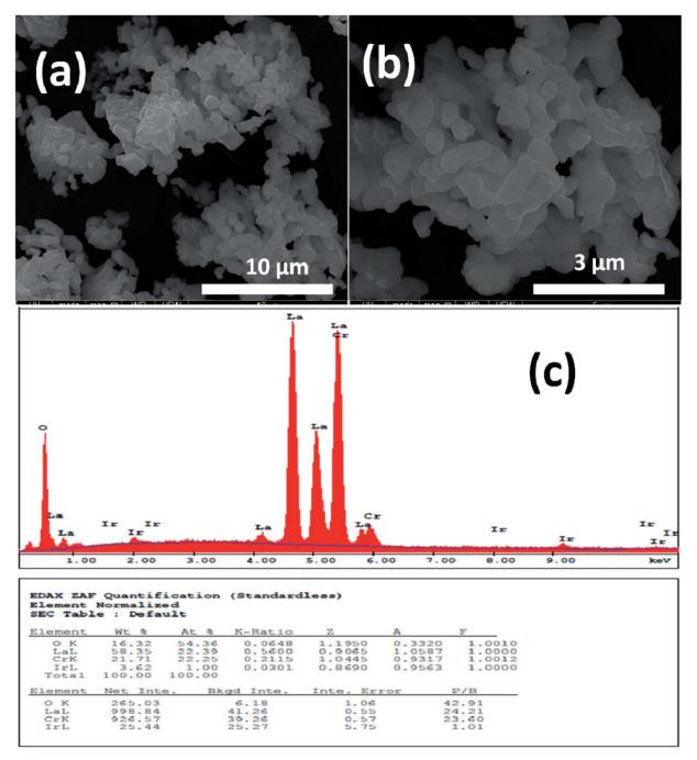
Fig. 2 (a and b) SEM images with different magnification (c) EDX analysis results for the 10% Ir doped LaCrO<sub>3</sub> powders, respectively.
