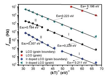
Fig. 9  $f_{\text{max}}$  versus (kT) $^{-1}$  plots of both LCO and Ir doped LCO samples. The solid lines represents the fits to the experimental data.
