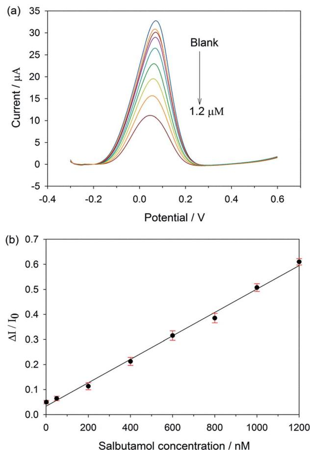
Fig. 3 (a) Differential pulse voltammograms of MIP/GP-PEDOT:PSS/SPCE recorded in 5 mM  $K_3[Fe(CN)_6]/K_4[Fe(CN)_6]$  after incubation in different concentrations of salbutamol, (b) calibration curve of the MIP/GP-PEDOT:PSS/SPCE. The error bars represent the standard deviation obtained from 6 independent measurements.
