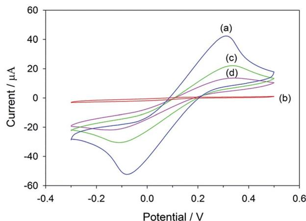
Fig. 1 Cyclic voltammograms of 5 mM  $\text{K}_3[\text{Fe}(\text{CN})_6]/\text{K}_4[\text{Fe}(\text{CN})_6]$  in 100 mM KCl at (a) graphene/PEDOT:PSS/SPCE, (b) MIP electrode before template removal, (c) MIP electrode after template removal and (d) MIP electrode after target rebinding.
