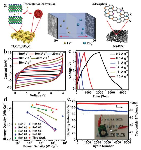
Fig. 5 (a) Schematic illustration of the charge-storage mechanisms for the  $Ti_3C_2T_x$ @Fe $_2O_3$ //NS-DPC LIC device. (b) CV curves and (c) chargedischarge curves of the  $Ti_3C_2T_x@Fe_2O_3//NS-DPC$  LIC device. (d) Ragone plots of the  $Ti_3C_2T_x@Fe_2O_3//NS-DPC$  LIC device and other previously reported devices. (e) Cycling stability of the  $Ti_3C_2T_x$ @Fe $_2O_3$ //NS-DPC device at a current density of 5 A  $g^{-1}$ ; the inset is a demonstration of the LIC device powering an LED.
