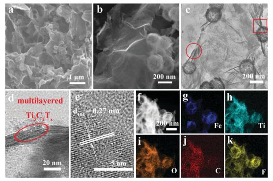
Fig. 2 (a and b) SEM images of the aerogel-like  $Ti_3C_2T_x@Fe_2O_3$  composite. (c) TEM image of the aerogel-like  $Ti_3C_2T_x@Fe_2O_3$  composite. (d and e) HRTEM images of the  $Ti_3C_2T_x@Fe_2O_3$  composite. The circle and box in panel (c) correspond to the HRTEM images for the selected area of panel (d) and (e), respectively. (f-k) Elemental mapping of the Ti<sub>3</sub>C<sub>2</sub>T<sub>x</sub>@Fe<sub>2</sub>O<sub>3</sub> composite.
