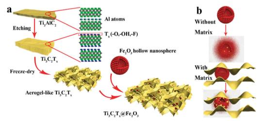
Scheme 1 (a) Schematic illustration of the synthesis procedure for the  $Ti_3C_2T_x@Fe_2O_3$  nanocomposite. (b) The mechanism of the MXene matrix protection in the Ti<sub>3</sub>C<sub>2</sub>T<sub>x</sub>@Fe<sub>2</sub>O<sub>3</sub> nanocomposite.
