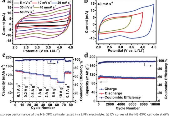
Fig. 4 Lithium storage performance of the NS-DPC cathode tested in a LiPF<sub>6</sub> electrolyte: (a) CV curves of the NS-DPC cathode at different scan rates. (b) CV curves of the NS-DPC cathode cycled within different potential windows at 40 mV s<sup>-1</sup>. (c) Rate performance of a NS-DPC cathode. (d) Cycling stability of a NS-DPC cathode at a current density of 5 A q<sup>-1</sup>.
