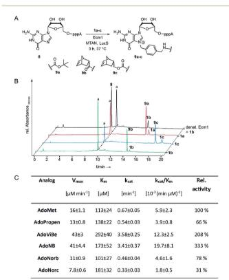
Fig. 1 (A) Enzymatic transfer of different functional moieties connected via benzyl linker to the mRNA cap analog GpppA. (B) HPLC chromatograms of enzymatic conversions after incubation at 37 °C for 3 h. Conditions: 300 μM 8, 20 mol% Ecm1 and 2 mM 1a-c. (C) Kinetic parameters from initial velocity measurements of Ecm1-catalyzed reactions with different co-substrates. Errors denote standard deviations of three independent experiments performed in duplicate.
