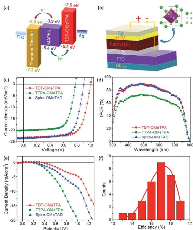
Fig. 4 (a) Energy level diagram for each layer of the PSC device based on the TDT-OMeTPA HTM. (b) Schematic of the planar PSC device. (c)  $J$ - $V$  curves under simulated 1.0 M sunlight, (d) IPCE curves, and (e)  $J$ - $V$  curves in the dark of PSC devices based on TDT-OMeTPA, TTPA-OMeTPA and Spiro-OMeTAD. (f) Histogram of 30 device PCEs based on the TDT-OMeTPA HTM.
