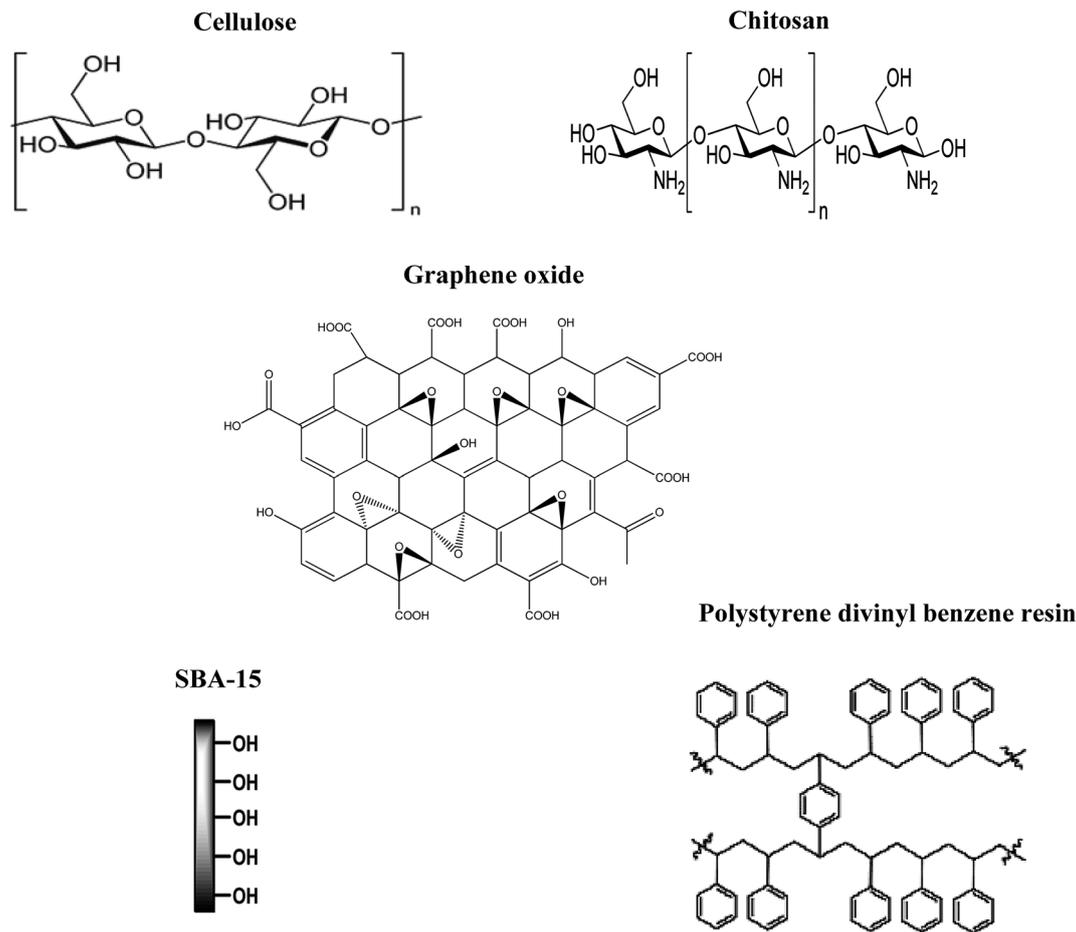
Fig. 2 Adsorbent materials with diverse functional groups.
