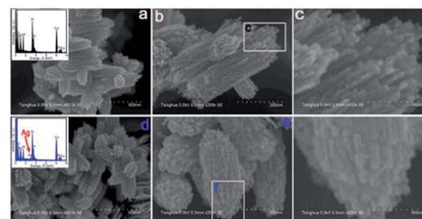
Fig. 22 (a) Low-, (b) medium-, and (c) high-magnification SEM images of  $\text{In}_2\text{O}_3/\text{ZnO}$  bundles, and (d) low-, (e) medium-, and (f) high-magnification SEM images of Ag-modified  $\text{In}_2\text{O}_3/\text{ZnO}$  bundles (this figure has been adapted from ref. 74 with permission from MDPI).
