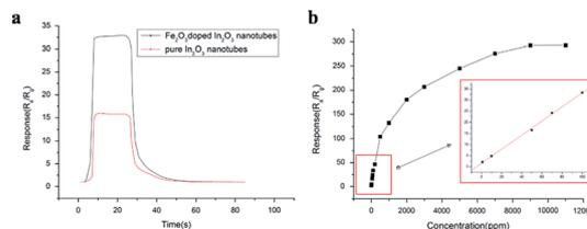
Fig. 21 (a) Response and recovery curves for  $\text{In}_2\text{O}_3$  and  $\text{Fe}_2\text{O}_3\text{-In}_2\text{O}_3$  nanotube gas sensors to 100 ppm formaldehyde (b) response of  $\text{Fe}_2\text{O}_3\text{-In}_2\text{O}_3$  nanotube sensors to different formaldehyde concentrations at  $250\text{ }^\circ\text{C}$ . The inset shows the calibration curve for 1–100 ppm (this figure has been adapted from ref. 73 with permission from Elsevier).
