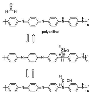
Fig. 19 Nucleophilic addition reaction between polyaniline and FA.
