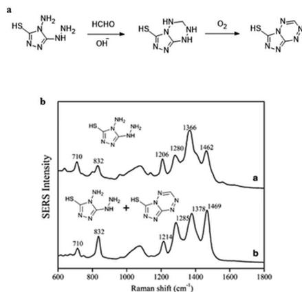
Fig. 14 (a) Derivative reaction of FA and AHMT under alkaline conditions. (b) SERS spectra of 500  $\mu\text{L}$  (a) AHMT in deionized water and (b) AHMT–MTT mixture in HCHO solution (this figure has been reproduced from ref. 70 with permission from Springer).
