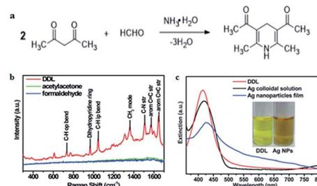
**Fig. 13** (a) Hantzsch reaction between FA and acetylacetone (acac), (b) Raman spectra of 10 mM DDL, acetylacetone, and FA at 457 nm excitation wavelength. (c) UV-vis spectra of DDL and AgNPs. The inset shows the photograph of DDL and AgNP solution under sunlight (this figure has been reproduced from ref. 69 with permission from RSC).
