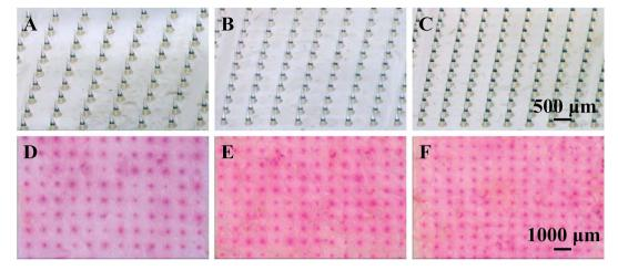
Fig. 4 Microscopic images showing the enlarging structure of the fabricated PLA MNs and the piercing effect of the MNs. (A-C) MN arrays with a height of 600 μm and different densities of (A) 144 MNs per cm<sup>2</sup>, (B) 196 MNs per cm<sup>2</sup> and (C) 256 MNs per cm<sup>2</sup>. (D-F) The porcine skin samples treated with MNs with different densities of (D) 144 MNs per cm<sup>2</sup>, (E) 196 MNs per cm<sup>2</sup> and (F) 256 MNs per cm<sup>2</sup>
