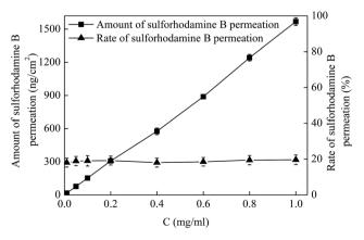
Fig. 5 The permeation profiles of sulforhodamine B with different concentrations across porcine skin samples treated with MNs. Each data point represents the average of 5 experiments. Standard deviation bars are shown.
