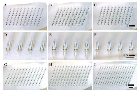
Fig. 1 Light micrograph of PLA MNs, as viewed from both (A–C, G–I) above and (D–F) side. (A, D)  $600~\mu m \times 100~MNs$  per cm<sup>2</sup>, (B, E)  $700~\mu m \times 196~MNs$  per cm<sup>2</sup>, (C, F)  $800~\mu m \times 100~MNs$  per cm<sup>2</sup>, (G)  $600~\mu m \times 144~MNs$  per cm<sup>2</sup>, (H)  $600~\mu m \times 196~MNs$  per cm<sup>2</sup>, (I)  $600~\mu m \times 256~MNs$  per cm<sup>2</sup>, where values indicate MN height  $\times$  array density.
