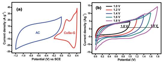
Fig. 7 (a) CV curves of AC and CoSe–G electrodes at the scan rate of 10 mV s $^{-1}$ ; (b) CV curves of ASC device in different potential windows at 10 mV s $^{-1}$ .
