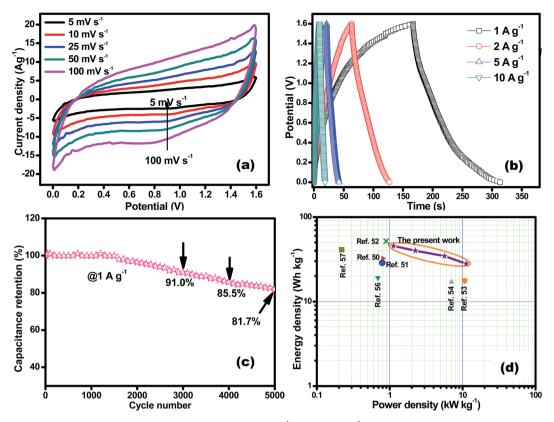
Fig. 8 (a) CV curves of ASC at different scan rates ranging from 5 mV s<sup>-1</sup> to 100 mV s<sup>-1</sup>; (b) galvanostatic charge–discharge curves of ASC at different current densities from 1 A g<sup>-1</sup> to 10 A g<sup>-1</sup>; (c) cycle stability of ASC device at constant current density of 1 A g<sup>-1</sup> upto 5000 charge–discharge cycles (d) Ragone plots of ASC device (energy density vs. power density).
