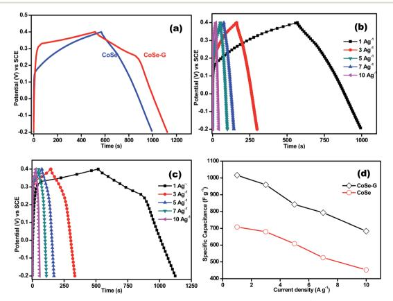
Fig. 5 (a) Galvanostatic charge–discharge of CoSe and CoSe–G at a constant current density of 1 A  $g^{-1}$ ; (b) galvanostatic charge–discharge studies of CoSe at different current densities; (c) galvanostatic charge–discharge studies of CoSe–G at different current densities; (d) specific capacitance of CoSe and CoSe–G electrodes as a function of different current densities.
