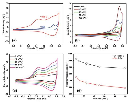
Fig. 4 (a) Cyclic voltammograms of CoSe and CoSe-G at 25 mV  $\rm s^{-1}$ ; (b) cyclic voltammograms of CoSe at different scan rates; (c) cyclic voltammograms of CoSe-G at different scan rates; (d) specific capacitance of CoSe and CoSe-G electrodes as a function of different scan rates.
