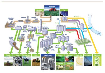
**Fig. 1** British Sugar Wissington biorefinery (Norfolk, UK), showing the main unit operations for sugar beet processing, to produce sucrose and a range of by-products including animal feed (from sugar beet pulp), bioethanol, vinasse, *etc.* (Reproduced with permission from British Sugar).
