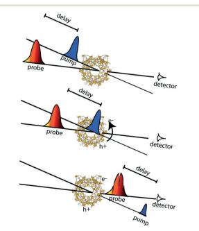
Fig. 4 Scheme of pump-probe experiment. In the middle panel, excitation of the framework by the pump beam takes place (charge separation is depicted in the figure). Systematic variation of the delay between pump and probe beams allows for recording transient absorption spectra with a time window from ~100 fs to several ns.
