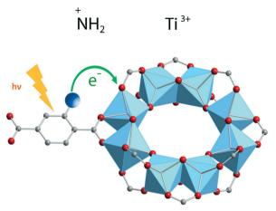
Fig. 6 Ligand-to-metal charge transfer (LMCT) and location of photogenerated charges in NH<sub>2</sub>-MIL-125(Ti).<sup>52</sup> Reproduced with permission from Wiley.
