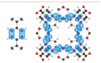
Fig. 2 Highest occupied states (HOCO) are localized on the aromatic organic group, while the lowest unoccupied states (LUCO) are localized on the octameric TiO<sub>2</sub> units for NH<sub>2</sub>-MIL-125(Ti).<sup>61</sup> Reproduced with permission from Wiley.
