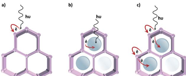
Fig. 7 Approaches for promoting photocatalytic activity in MOFs: a) the organic linker harvests the light and LMCT is promoted; b) the MOF is used as a container of a light absorbing catalyst; c) charge transfer occurs between the MOF and the encapsulated catalyst.
