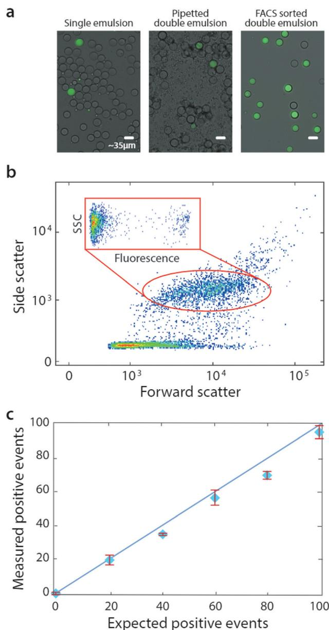
**Fig. 3** Bulk dispersal allows accurate droplet quantitation over a range of concentrations. Microfluidic droplets are generated (a, left) and bulk double emulsified into aqueous carrier *via* pipetting (a, middle), followed by analysis and sorting with flow cytometry (a, right). During FACS, scattering and fluorescence are measured (b). The number of detected positive droplets scales with the number of positives added to the single emulsion (c).
