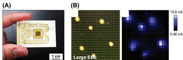
**Fig. 9** LSI-based electrochemical device. (A) Device image.<sup>63</sup> (B) Real-time monitoring of ALP activity of EBs on the device.<sup>58</sup> Reproduced with permission from Elsevier ©2013 and 2016.
