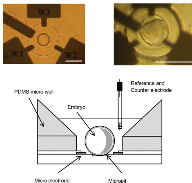
**Fig. 8** Chip device with three platinum working electrodes, a circular SiO<sub>2</sub> insulator layer, and a cylindrical micropit for evaluation of respiratory activity.<sup>45</sup> Scale bars: 100 μm. Reproduced with permission from Elsevier ©2011.
