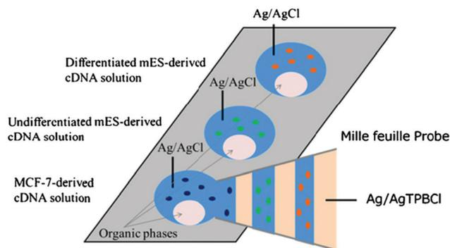
**Fig. 7** Mille-feuille probe containing the lamination of the aqueous and organic phases under voltage control for simultaneous detection of multiple cDNAs collected with the mille-feuille probe.<sup>37</sup> Reproduced with permission from Springer ©2017.
