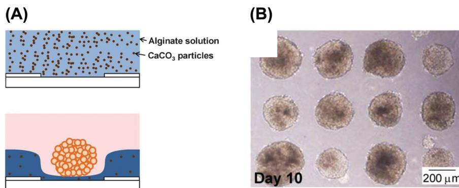
**Fig. 13** Electrodeposited hydrogel microwells used for 3D cell culturing. (A) Fabrication scheme. (B) HepG2 spheroids in the microwells.<sup>81</sup> Reproduced with permission from the Royal Society of Chemistry ©2013.
