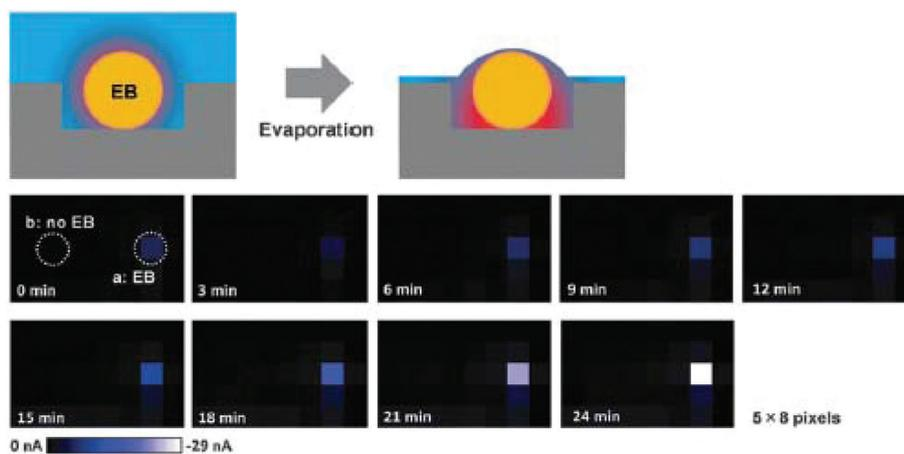
**Fig. 11** Evaporation-based electrochemical detection of ALP activity in EBs.<sup>66</sup> Illustrations of the outline (top row). Time-course analyses of electrochemical images of an EB (middle and bottom row). Redox compounds were accumulated as the incubation time increased. Reproduced from the Royal Society of Chemistry ©2012.
