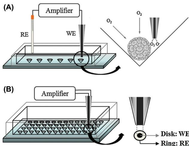
**Fig. 3** Electrochemical detection of O<sub>2</sub> consumption by 3D cultured cells using SECM.<sup>14</sup> (A) Conventional SECM system, working (WE) and reference (RE) electrodes are inserted into a solution, and 3D cultured cells are trapped in a microwell. (B) Probe devices containing both working (WE) and reference electrodes (RE) for simplifying the detection procedure. Reproduced with permission from Elsevier ©2012.
