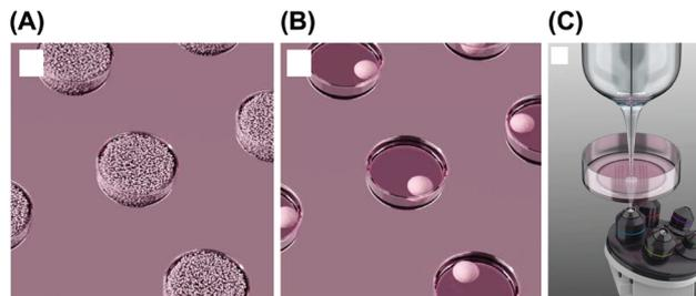
**Fig. 4** The concept of SECM-based assays for microtissues fabricated in a microwell array.<sup>15</sup> (A) Cells are seeded and centrifuged to set them into the microwells. (B) Cell aggregates form after culture. (C) SECM measurements are performed for the cell culture arrays. Reproduced from Public Library of Science ©2014.
