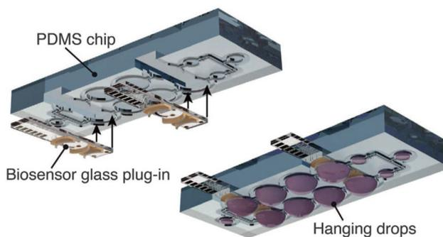
**Fig. 10** Design of the droplet array microfluidic device with enzyme-modified electrodes.<sup>73</sup> Reproduced from Springer Nature ©2016.
