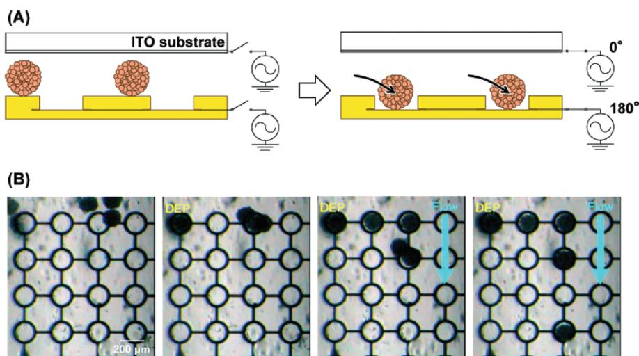
**Fig. 12** Manipulation of EBs using DEP. (A) Scheme. (B) Optical images of the EBs on the device during DEP and fluidic manipulations.<sup>70</sup> Reproduced with permission from the Royal Society of Chemistry ©2015.
