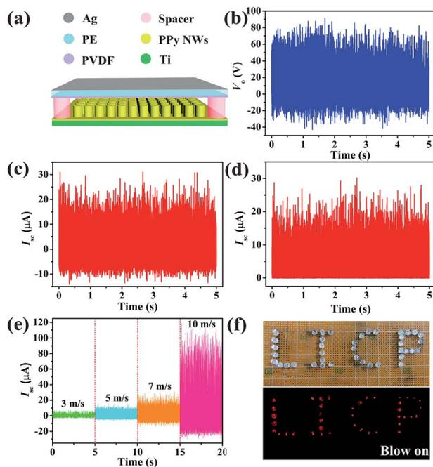
Fig. 5 (a) Device structure of the designed PPy NW-based W-TENG. (b)  $V_o$ , (c)  $I_{sc}$  and (d) the rectified  $I_{sc}$  at a wind speed of  $7 \text{ m s}^{-1}$  (on the scale of 4 BF). (e) The  $I_{sc}$  at different wind speeds from  $3 \text{ m s}^{-1}$  (2 BF) to  $10 \text{ m s}^{-1}$  (5 BF). (f) Photographs of 40 LEDs before and after being powered by the W-TENG.
