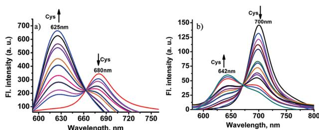
Fig. 4 (a) Fluorescence spectra of **CHMC1** (5  $\mu\text{M}$ ) in the aqueous buffer in the presence of a high concentration range of Cys (35–500  $\mu\text{M}$ ), excitation at 550 nm; (b) fluorescence spectra of the probe **CHMC2** (5  $\mu\text{M}$ ) in aqueous buffer in the presence of a high concentration range of Cys (35–500  $\mu\text{M}$ ), excitation at 550 nm.
