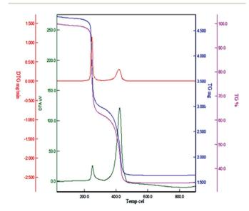
Fig. 4 TGA curve of Cu(II) immobilized on Fe<sub>3</sub>O<sub>4</sub>@SiO<sub>2</sub>@L-arginine.
