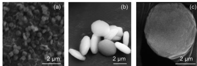
Fig. 2 SEM micrographs of (a) Sigma1-315-S (b) Sigma1-315-M (c) Sigma1-315-L with  $\text{SiO}_2/\text{Al}_2\text{O}_3 = 315$ .
