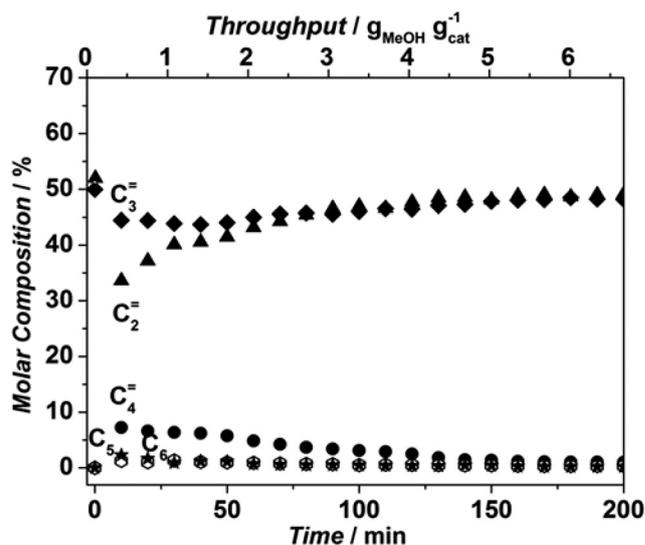
Fig. 11 Product distribution in co-feeding C<sub>2</sub>H<sub>4</sub> and C<sub>3</sub>H<sub>6</sub> in the presence of water over Sigma1-315-S at 450 °C.
