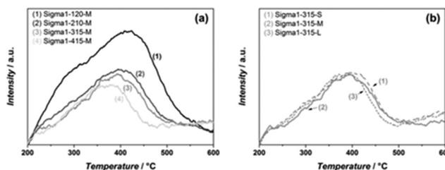
Fig. 3  $\text{NH}_3$  TPD profiles of Sigma-1 zeolites with different  $\text{SiO}_2/\text{Al}_2\text{O}_3$  ratio and medium crystal size (a), and of different crystal sizes with  $\text{SiO}_2/\text{Al}_2\text{O}_3$  ratio = 315 (b).
