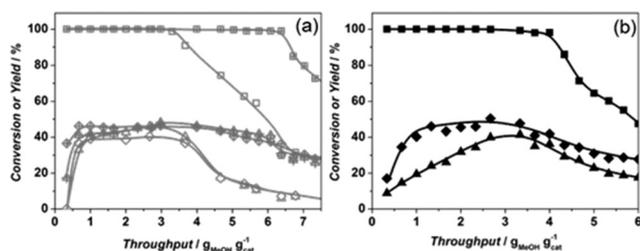
Fig. 8 Methanol conversion (■), ethylene (▲) and propylene (◆) yields of (a) Sigma1-315-S (□, △, ◇) and Sigma1-315-S-m (■, ▲, ◆); (b) ZSM-58 (■, ▲, ◆) (SiO<sub>2</sub>/Al<sub>2</sub>O<sub>3</sub> = 110, 0.6–1.8 μm) at 450 °C and standard operation conditions.
