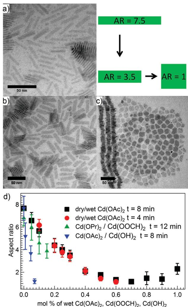
Fig. 2 TEM images of samples (a) NPL-1, (b) NPL-6, (c) and NPL-10 illustrating the aspect ratio control. (d) Plot of the CdSe NPL aspect ratio versus the molar percentage of Cd(OAc)<sub>2</sub>·2H<sub>2</sub>O, Cd(OOCH)<sub>2</sub>, and Cd(OH)<sub>2</sub> precursors, respectively.
