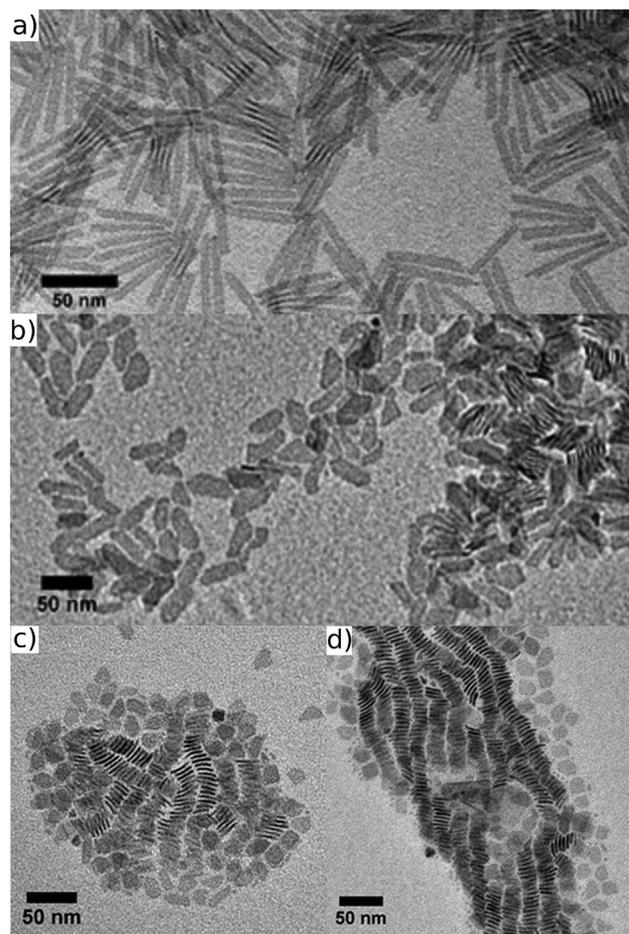
Fig. 1 (a) TEM image of 4.5 mL of CdSe NPLs synthesized using dry Cd(OAc)<sub>2</sub>. (b) TEM image of 4.5 mL of CdSe NPLs synthesized using Cd(OAc)<sub>2</sub>·2H<sub>2</sub>O. (c) TEM image of 4.5 mL of CdSe NPLs synthesized using dry Cd(OAc)<sub>2</sub> and 20 μL of water. (d) TEM image of 4.5 mL of CdSe NPLs synthesized using 93 mol% dry Cd(OAc)<sub>2</sub> and 7 mol% Cd(OH)<sub>2</sub>.
