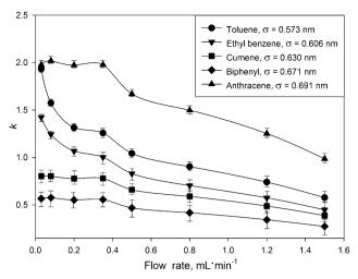
Fig. 1 Influence of the mobile phase flow rate on the retention factors for model compounds on the UiO-66@SiO2 column. Mobile phase n-hexane, 25 °C, sample volume 2  $\mu$ L of 100  $\mu$ g mL<sup>-1</sup> solutes in n-hexane. Kinetic diameter ( $\sigma$ , nm) for each analyte was calculated as suggested by Jae et al. 16 using critical constants from. 17
