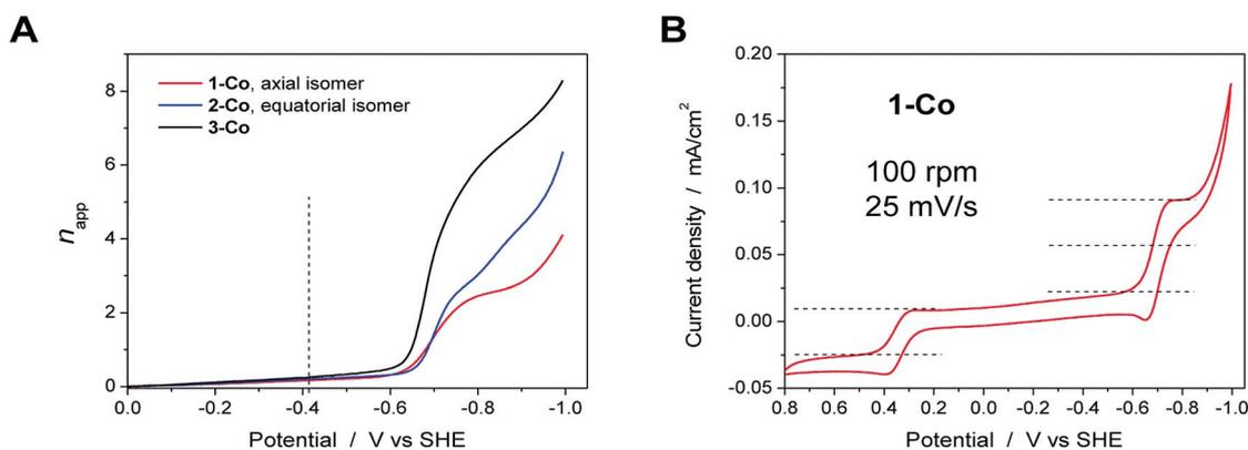
Fig. 7 A. Comparison of  $n_{app}$  vs. applied potential for catalysts **1-Co** (red), **2-Co** (blue), and **3-Co** (black) based on steady-state voltammograms in Fig. 6 (bottom). The vertical dashed line denotes the thermodynamic potential for water reduction at pH 7. B. Steady-state voltammogram of catalyst **1-Co** at 100 rpm, 25 mV s<sup>-1</sup>.
