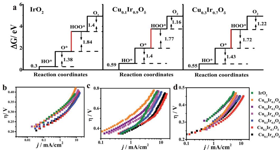
Fig. 7 (a) Standard free energy diagram for the OER in  $\text{IrO}_2$ ,  $\text{Cu}_{0.1}\text{Ir}_{0.9}\text{O}_8$  and  $\text{Cu}_{0.3}\text{Ir}_{0.7}\text{O}_8$ . (b–d) Tafel plots in acidic, neutral and basic solutions, respectively. The curves are iR-corrected in the acidic ( $\sim 18 \Omega$ ), neutral ( $\sim 15 \Omega$ ) and basic ( $\sim 28 \Omega$ ) solutions, respectively. The catalyst mass loading was  $\sim 0.2 \text{ mg cm}^{-2}$  for all electrodes.
